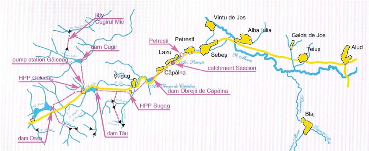
Fig. 1 – Sebes complex hydro energetic scheme
