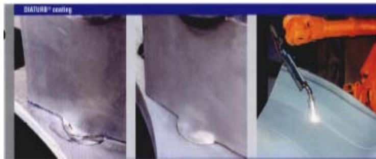
Fig 20 Coating on Francis components
